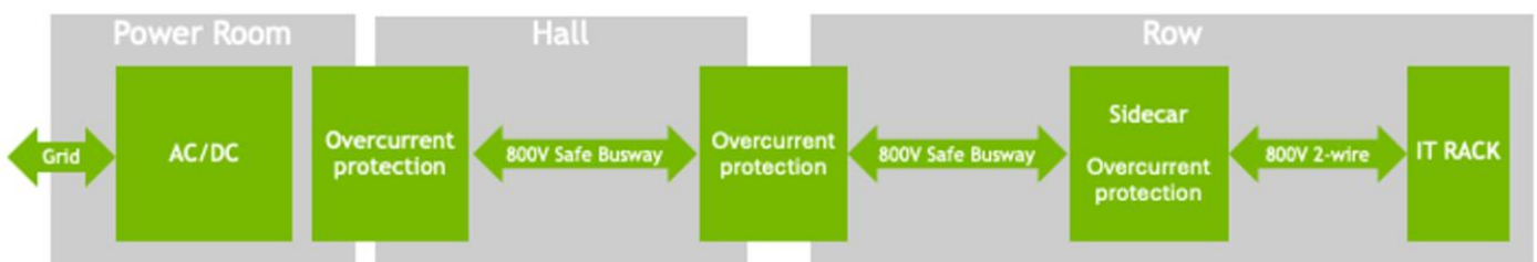
Figure 2. NVIDIA 800 VDC architecture minimizes energy conversions.
